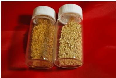
Unprocessed dried distiller's grain is shown on the left, and processed DDG is on the right.
